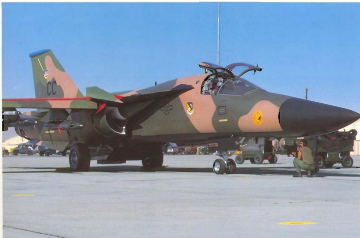
Left A Cannon-based F-111 carrying a Cubic Corporation ACMI pod for transmission of aerial data to computers on the ground. ACMI stands for Air Combat Manoeuvring Instrumentation; with this system an aerial engagement can be viewed in computer simulation on the ground or taped for later debrief by the pilots
