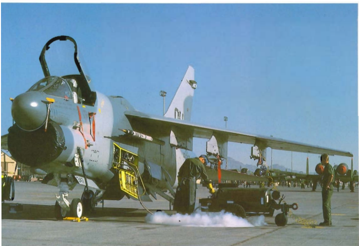
A-7Ds of the 112th TFS, 180th TFG, Ohio ANG, take on liquid oxygen at Gunsmoke 1987
