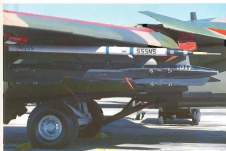
Left A Cannon-based F-111 carrying a Cubic Corporation ACMI pod for transmission of aerial data to computers on the ground. ACMI stands for Air Combat Manoeuvring Instrumentation; with this system an aerial engagement can be viewed in computer simulation on the ground or taped for later debrief by the pilots
