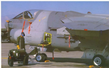
A-7Ds of the 112th TFS, 180th TFG, Ohio ANG, take on liquid oxygen at Gunsmoke 1987
