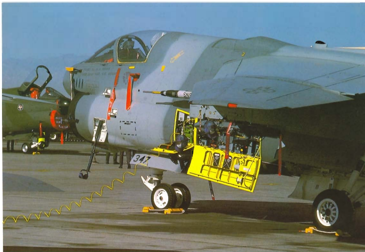
The A-7D has 35 access panels, 90 per cent of which can be reached without an aircraft stand. US Air Force units gave up their A-7s to the Air Guard following the introduction of the Fairchild A-10A Thunderbolt II in the mid-1980s
