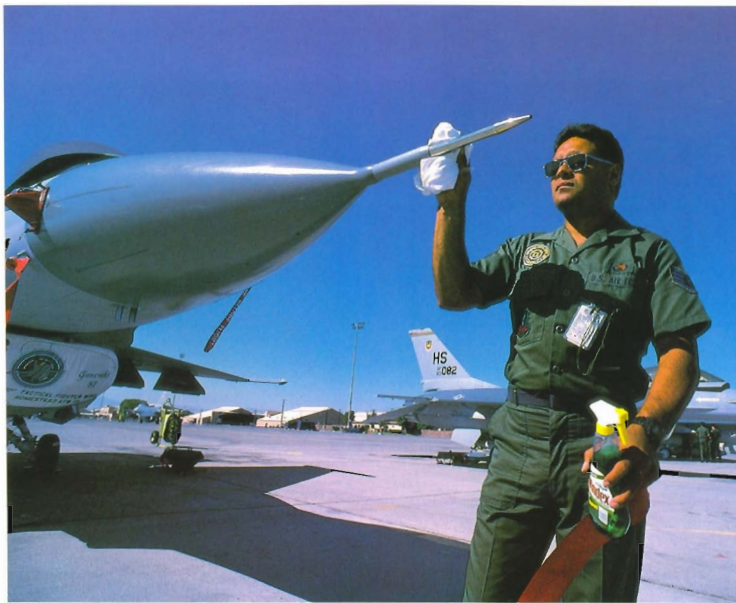
The pitot head of a 31st TFW F-16 gets a final polish before a Gunsmoke inspection
