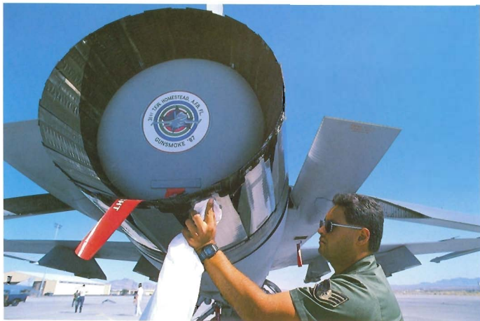
From front to back: the same polisher shines the con/di nozzle of the P&W F100-200 turbofan
