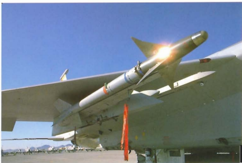
Right Close-up of a captive Sidewinder missile and a Copic data transmitter (nearest camera) fitted to an F-18. The aircraft has four missile stations for the semi-conformal carriage of the medium-range radar guided Sparrow air-to-air missile; one of the stations can be seen under the intake
